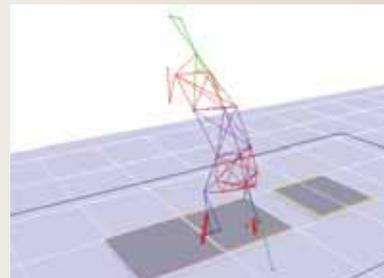
**Figure 2b.** Documentation of reflective marker recording was performed using Cortex software. Ground reaction forces were also recorded (red arrows).
